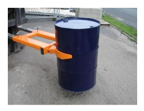
If your drums are damaged, open topped, or empty you will experience difficulty lifting with this attachment. The IRG range are best suited for lifting this variety including straight sides drums.
