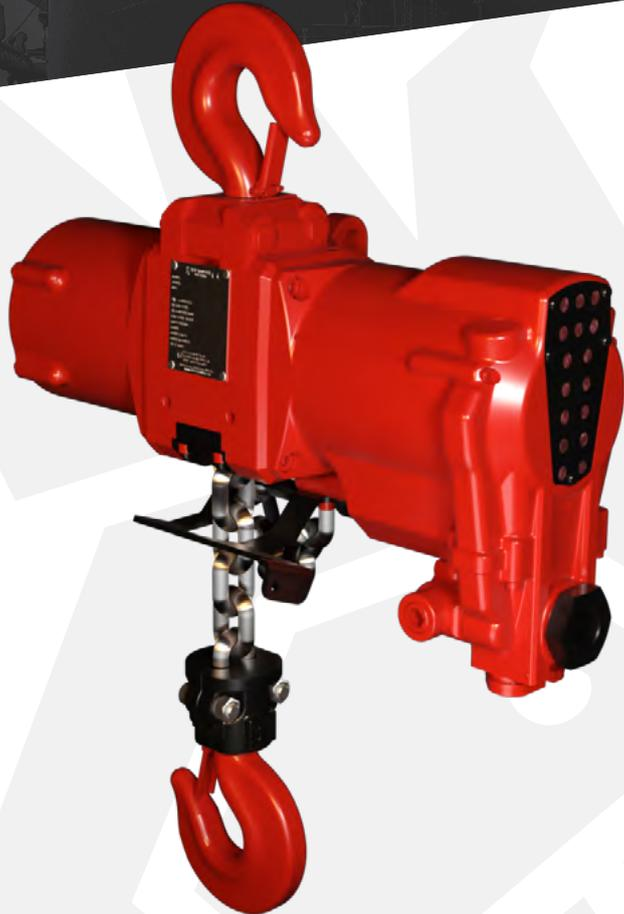
The new **Red Rooster Lifting** TMH series air hoists have the highest lifting speed with the lowest headroom on the hoist market. With the high M4 classification of mechanism (ISO 4301-1) this high speed air hoist is extremely durable and will guarantee the continuity of your process. The TMH hoists are designed to operate at full lifting capacity with an air pressure from 4 – 6.3 bar. For full speed operation the hoist air pressure should be 6.3 bar.
