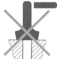
9. All fittings connected to the STARPOINT-eyenut should be free moving. When connecting and disconnecting the lifting means (sling chain) pinches and impacts should be avoided. Damage of the lifting means caused by sharp edges should be avoided as well.
