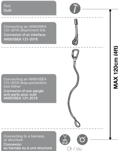
**6. Installing the attachment link on the tool**
