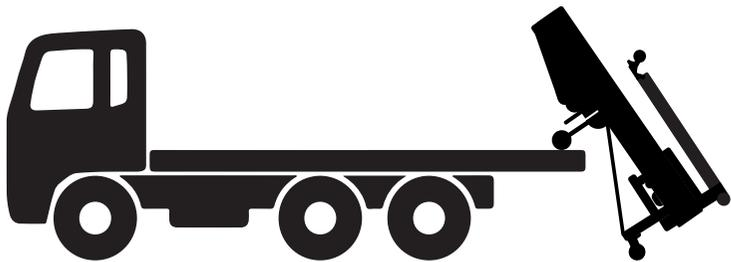
9. Use a minimum of 2 straps or chains to secure the machine to the flatbed of the vehicle or trailer. **If laying the machine down on the vehicle or trailer, ensure that the straps are placed over the mast, as putting them over the front legs could cause damage to the machine.**
