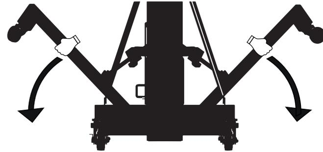
5. Lower the steering handle/loading wheel assembly by removing the retaining pin, lowering, and then locking in place with the retaining pin.
