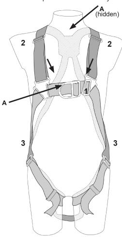
Harnesses are made from polyamide and polyester, with steel and aluminium alloy fittings.
