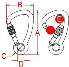
Oval carabiner carbon steel, wide-opening. High load of 40 kN. Ideal for heavy duty applications and for connection to structural anchors, lifelines, etc.
