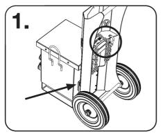
Butt the rubber pads against the transformer and unclip the hooks from the holes on the back of the T-Kart.
