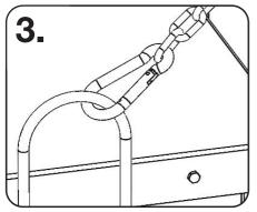
Use the clip hooks to attach both chains to the hoops/handles of the transformer.
