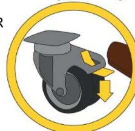
Brakes must be Locked
