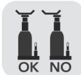
Jack Saddle axis in line (no offset load)
