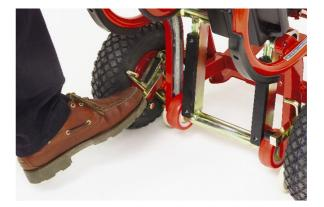
Turning further by foot or hand to neutral position. (Then the middle wheel of the 3 brake wheels is stopped by a cam on the frame- when turning the brake anticlockwise.)
