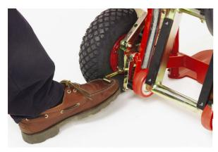
Switching the brake back to neutral position by foot or by hand.
