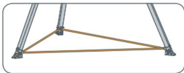
Grasp the tail end of the webbing exiting each adjustment buckle and pull, tightening the strap to remove any slack. Tighten all three straps evenly to maintain a triangular foot and ensure the TRIBUS is set up with the legs at the approved angle (see 7.)
