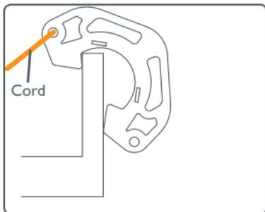
Ensure the edge being protected is of sufficient strength to support the rope running over it and the foreseeable maximum load. Use the cords to secure the Edge Guard to the structure.
