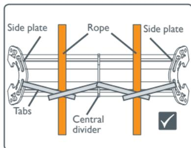
The positioning of the rope on the Edge Guard may be affected by rope deviations below the Edge Guard and changes in work position while carrying out the work task; ensure that the Edge Guard is positioned accordingly before beginning work. Beware, the greater the distance between the Edge Guard and the anchor point, the greater the potential for lateral movement of the rope.
