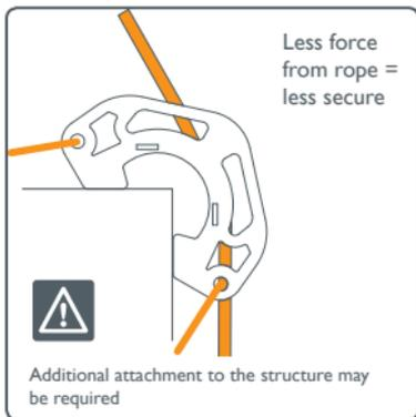
The Edge Guard must be positioned so that the rope runs over the centre of the Edge Guard, and does not lift out or become trapped against the side plates. Use the Velcro tabs to help keep the rope in place.
