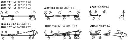
ATTENTION! The energy absorbers can be equipped only with certified (according to EN362) connectors
