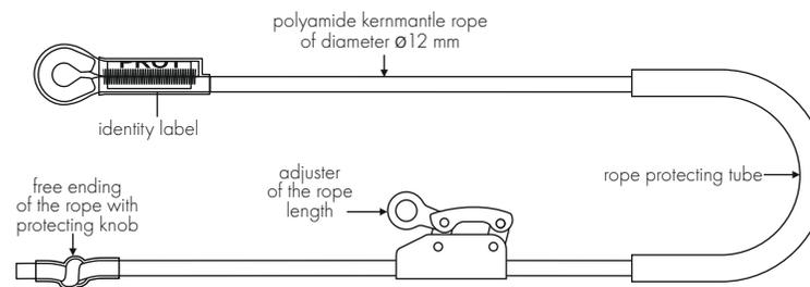
Using the work positioning device PROT-2 in connection with connectors must be compatible with their instructions and obligatory standard EN 362.
