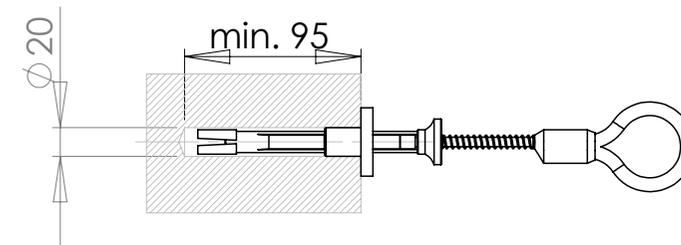
3. Make sure that sliders are fastened in the hole by pulling device into "X" direction.
