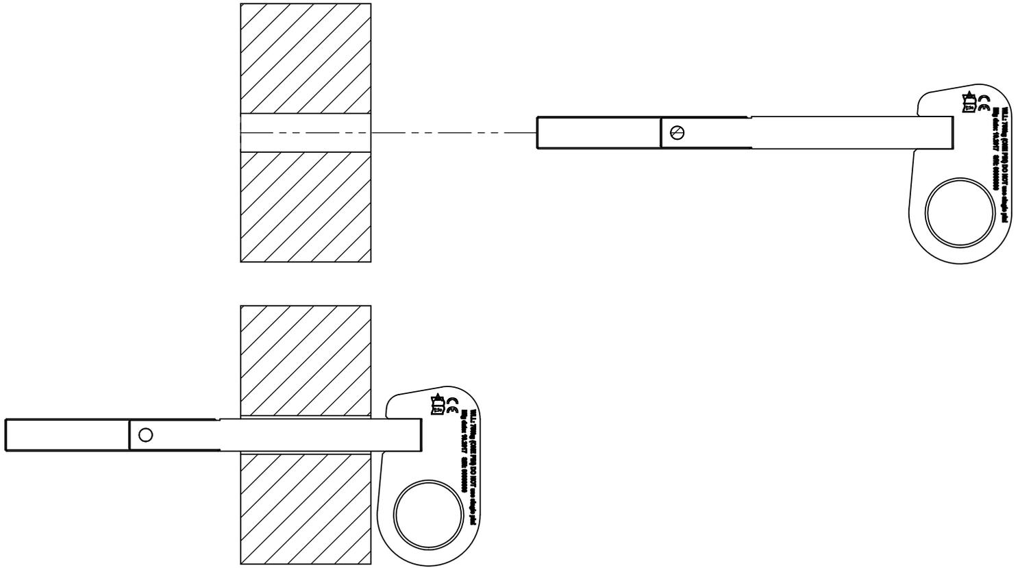
3. Rotate lifting pin 180°. Pawl should be locked.
