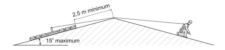
When used on steel cladded roofs up to 15 ° pitch always place the Mobile Man Anchor on the opposite pitch to the one you are working on. Always position the Mobile Man Anchor a minimum of 2.5m from the ridge on the opposite pitch. When working on the verge detail remember to position the Mobile Man Anchor at least 2.5m from the verge and only work opposite the Mobile Man Anchor in order to avoid the pendulum effect down the fa\u+00e7ade of the building.
