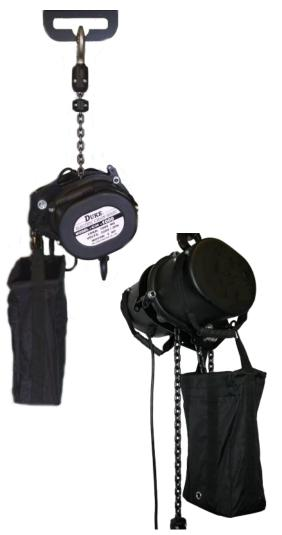
LiftinGear Duke Electric Inversion / Standard use Hoist
